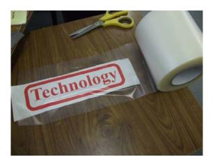
Use the squeegee to attach the application tape firmly to the sign.
