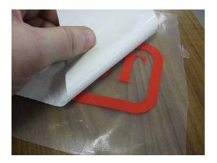
Put the vinyl on the substrate and use the squeegee to attach it firmly,
