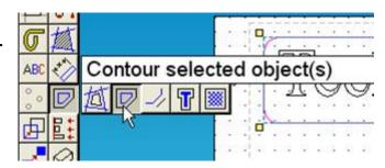
Set the contour spacing to 8mm and select **Outside** from the dialog box. This will draw an 8mm line around the outside of the existing outline.
