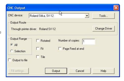
Before selecting Output, ensure that the Vinyl is loaded into the Stika from the front and that the blade is set to the correct depth.
